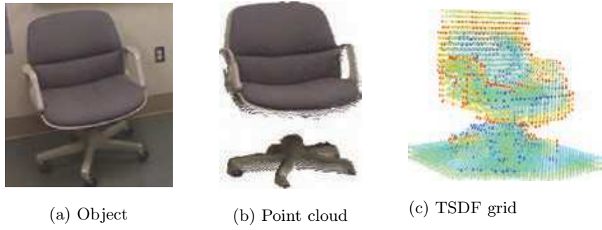
Figure 2: TSDF representation proposed by Song and Xiao as shown in their paper [3]. An object (a) is captured by a range sensor as a point cloud (b) and then a TSDF grid is generated (red indicates the voxel is in front of surfaces and blue indicates the voxel is behind the surface; the intensity of the color represents the TSDF value).
