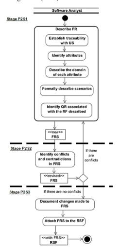
Fig. 3. Activity diagram (1) UML 2.X associated with Phase 2 "Detailed specification of functional".
