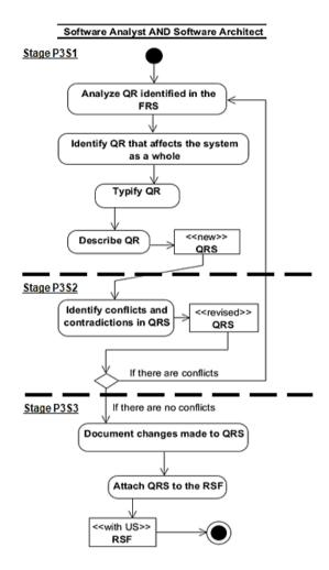
Fig. 4. UML 2.X activity diagram associated with Phase 3 "Detailed specification of quality requirements".
